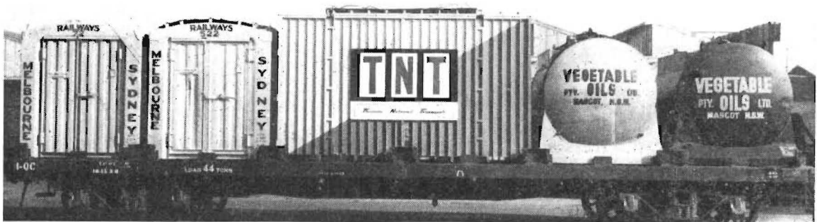
L.C.L. containers on specially designed QC wagon.
